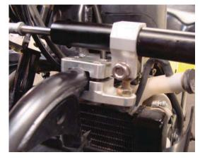
Next mount the square clamp on the frame rail in the desired location making sure to evenly torque the mounting hardware to 30 foot pounds.
